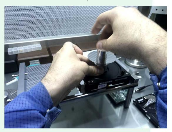
9) Turn around the Platter Container System (to clean the other side of the platter).
