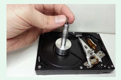
4) Screw in the screw (not supplied in this kit) firmly onto the motor shaft (this prevents it from vibrating).
